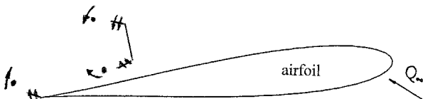
Fig. 4 Separated flow model for airfoil with base-vented spoiler.
